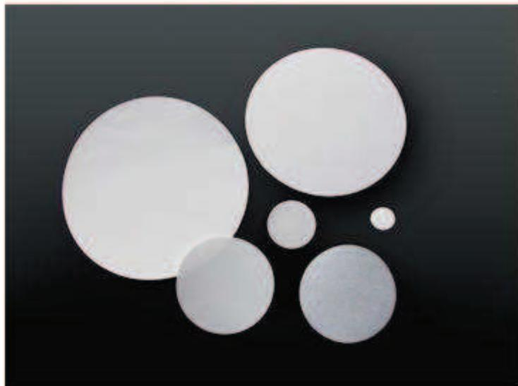
Membrane filters or "membranes" are microporous films with specific pore size ratings. Membranes retain particles and microorganisms that exceed their pore ratings by acting as a physical barrier and capturing such particles on the surface of the membrane.
